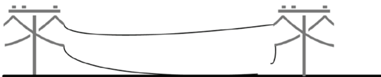
Figure 2: Downed Broken Conductor
