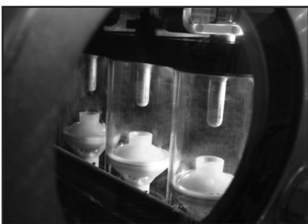
▲ Three phase visible position of contacts.
