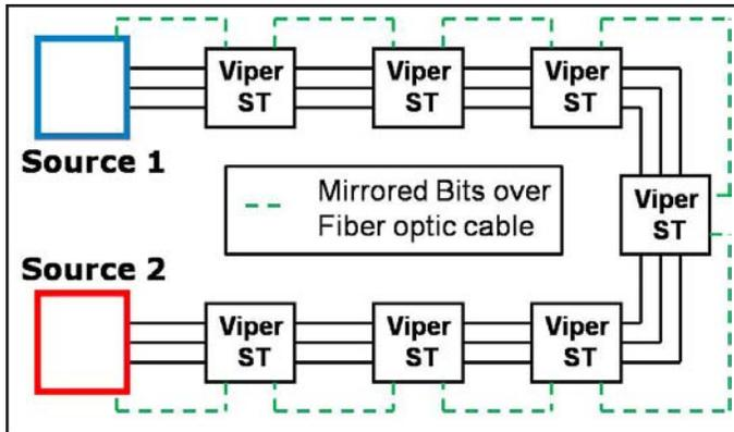
Diagram 1: Single Phase Tripping, Closed Loop
