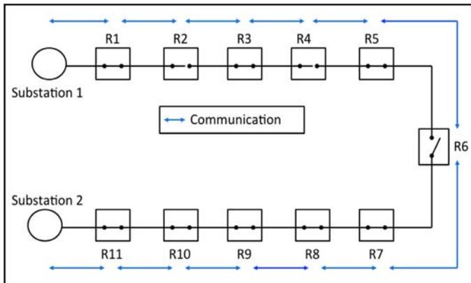
Diagram 2: Three Phase Tripping, Open Loop
